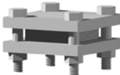
Figure 2 Torque Plates
