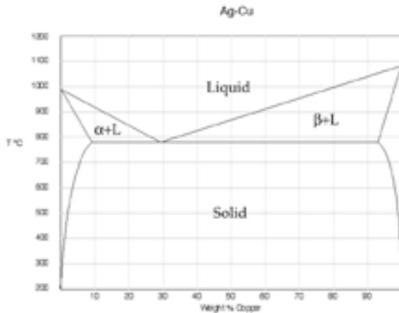
eutectic during the lamination process, the metals will tend to form the eutectic alloy as they are attempting to reach equilibrium. The alloy at the interface between layers will lose cohesion and the remaining sheets will slip and slide in the liquid. This almost always results in having to scrap that billet. This makes learning to read phase diagrams an important
